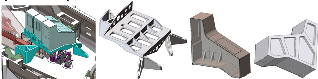
Figure 12. Auxiliary optical bench and J, K, H channel housing details.
