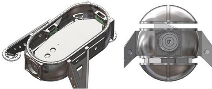
Figure 7. Optical bench suspended in cryostat midsection and exploded view of cryostat hatches.
