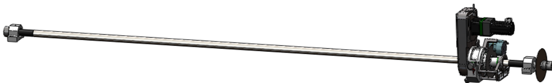
Figure 3. CAD illustration of the UX roller screw drive system (track drive motor and screw bearing mounts not shown).
